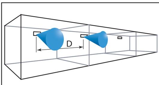
Figure 20. A large room ventilated by several wall diffusers
