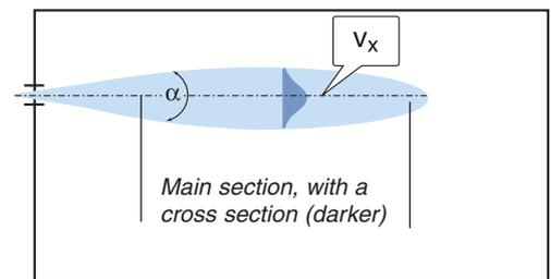
Figure 9. The main section of the air stream, the centre velocity  $v_x$  and discharge angle.
