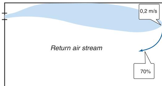
Figure 15. Return air stream with a wall-mounted diffuser
