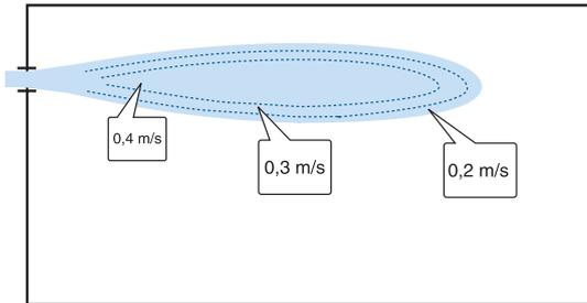
Figure 11. The different isovels of an air stream
