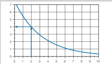
The difference between the total sound level and the sound level of the supply system is 2 dB. The diagram indicates that 4 dB must be deducted from the total level.
