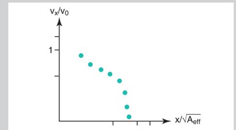
Using the values obtained from the main section of the air stream, a tangent (angle coefficient) is drawn at an angle of -1 (45°).
