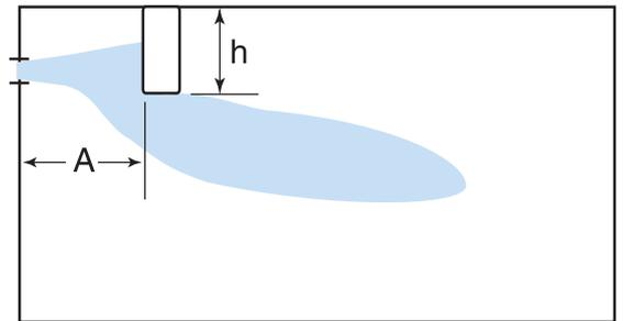
Figure 17. Minimum distance to an obstacle
