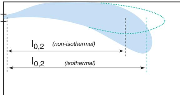
Figure 23. The difference between the throws of isothermal and non-isothermal air streams.
