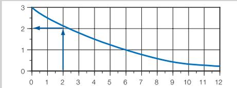
The difference between the sound levels is 2 dB and, according to the diagram, 2 dB must be added to the highest level.
