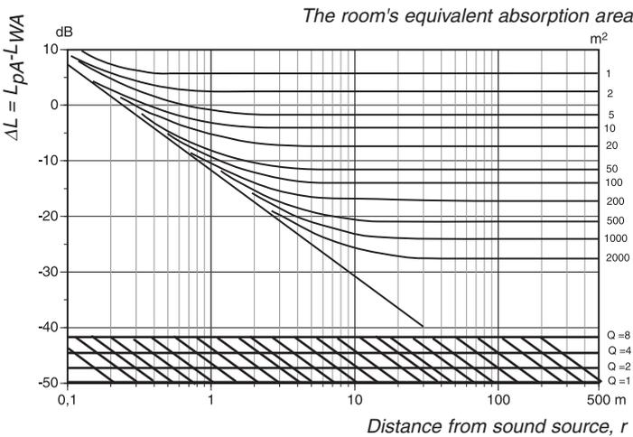
Figure 3. Diagram for estimating the sound pressure level
