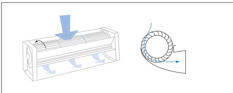
Figure 27. The air flow through a cross-flow fan
