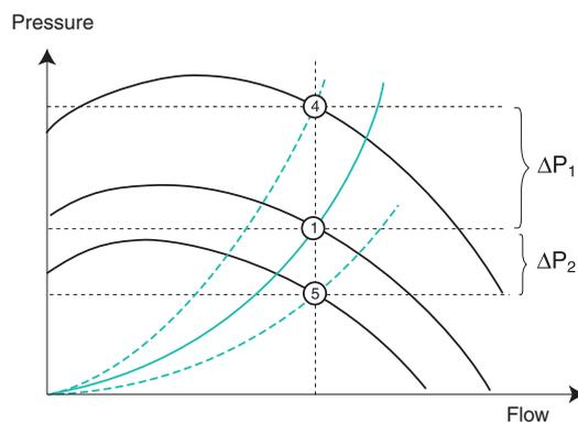
Figure 31. Pressure differences at different rotational speeds
