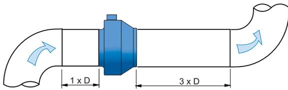
Figure 34. Correctly installed duct fan
