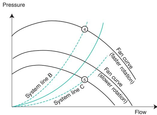
Figure 30. Increase or reduction of the fan speed
