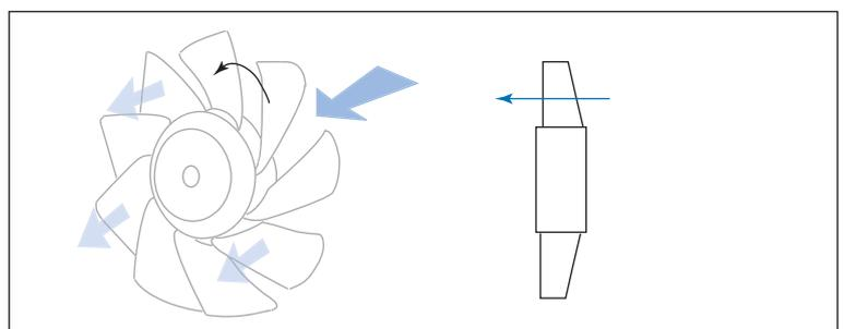
Figure 25. The air flow through an axial fan
