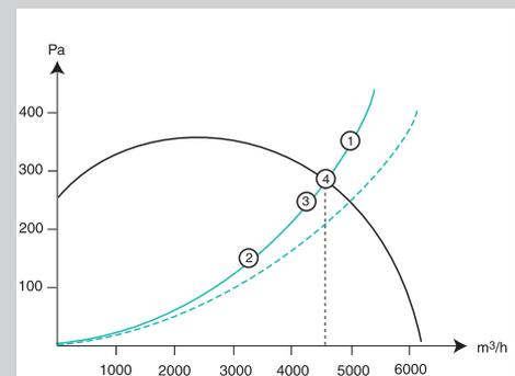
The new working point (4) is located at the intersection between the fan curve and the new system line.
