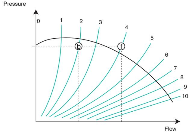
Figure 32. System lines (0-10) in a fan diagram
