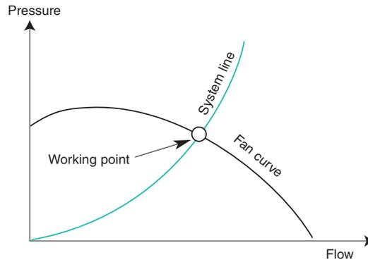
Figure 28. Curves in a typical fan diagram
