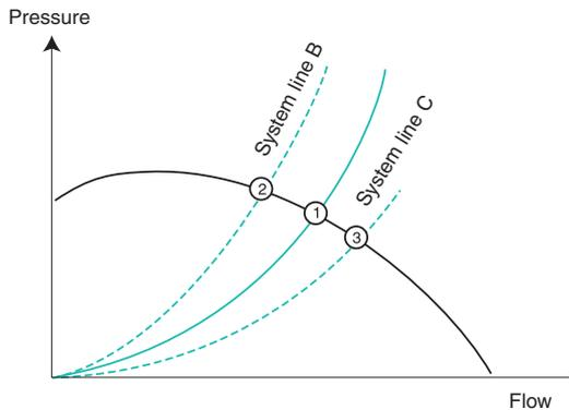
Figure 29. Changes in pressure give rise to new system lines
