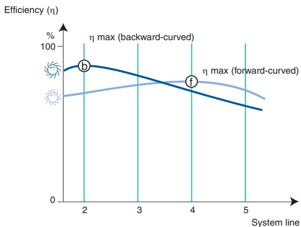
Figure 33. Efficiency values for the same size of radial fan with backward-curved and forward-curved blades respectively
